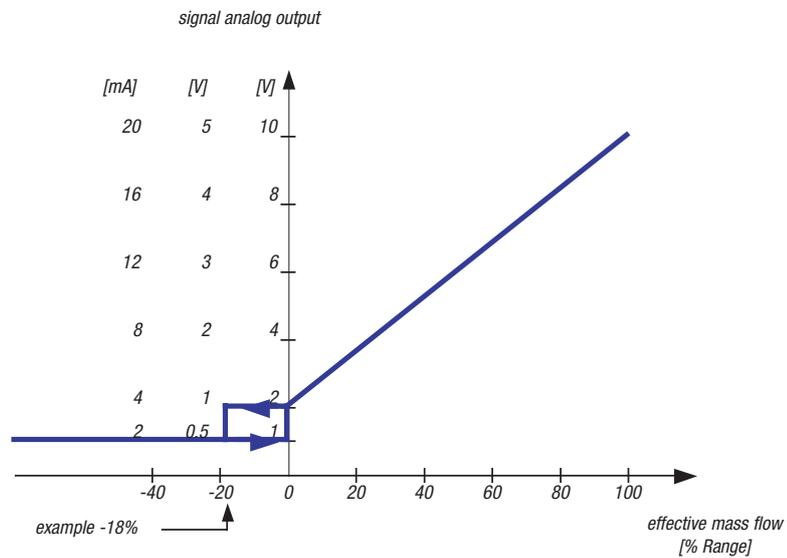
If the condition for setting alarm flag #1 is fulfilled, the analog output is set to half the value of the minimum output value.
