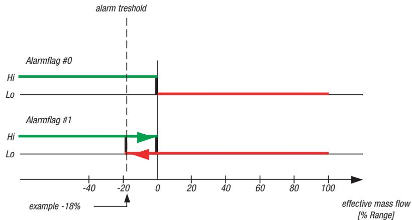
Here, the alarm threshold that can be adjusted by the user influences the hysteresis behaviour of the alarm flag #1.
